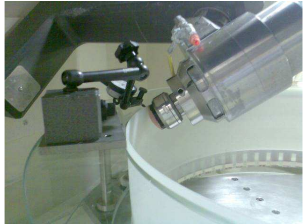
Fig. 14: Particular of the Bonnet polishing tool during one of first grolishing tests, performed to evaluate the suitability of the SSS jig as interface to the polishing machine.
