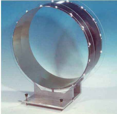
Fig. 5: Prototype shell realized in SiC by epoxy replication technique and successfully X-ray calibrated. The diameter is 600 mm, the height 200 mm and the thickness 2 mm.
